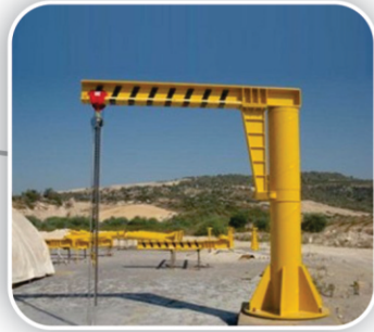
Pig Handling Crane (Jib Crane)
